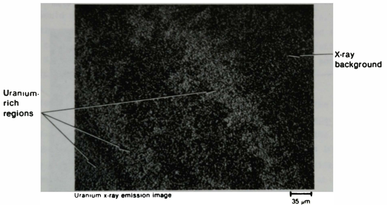
Figure 18. Multiple forms of U, Zr, and O segregation upon cooldown of a heterogeneous melt near the fuel-cladding interface in Particle 1E.
