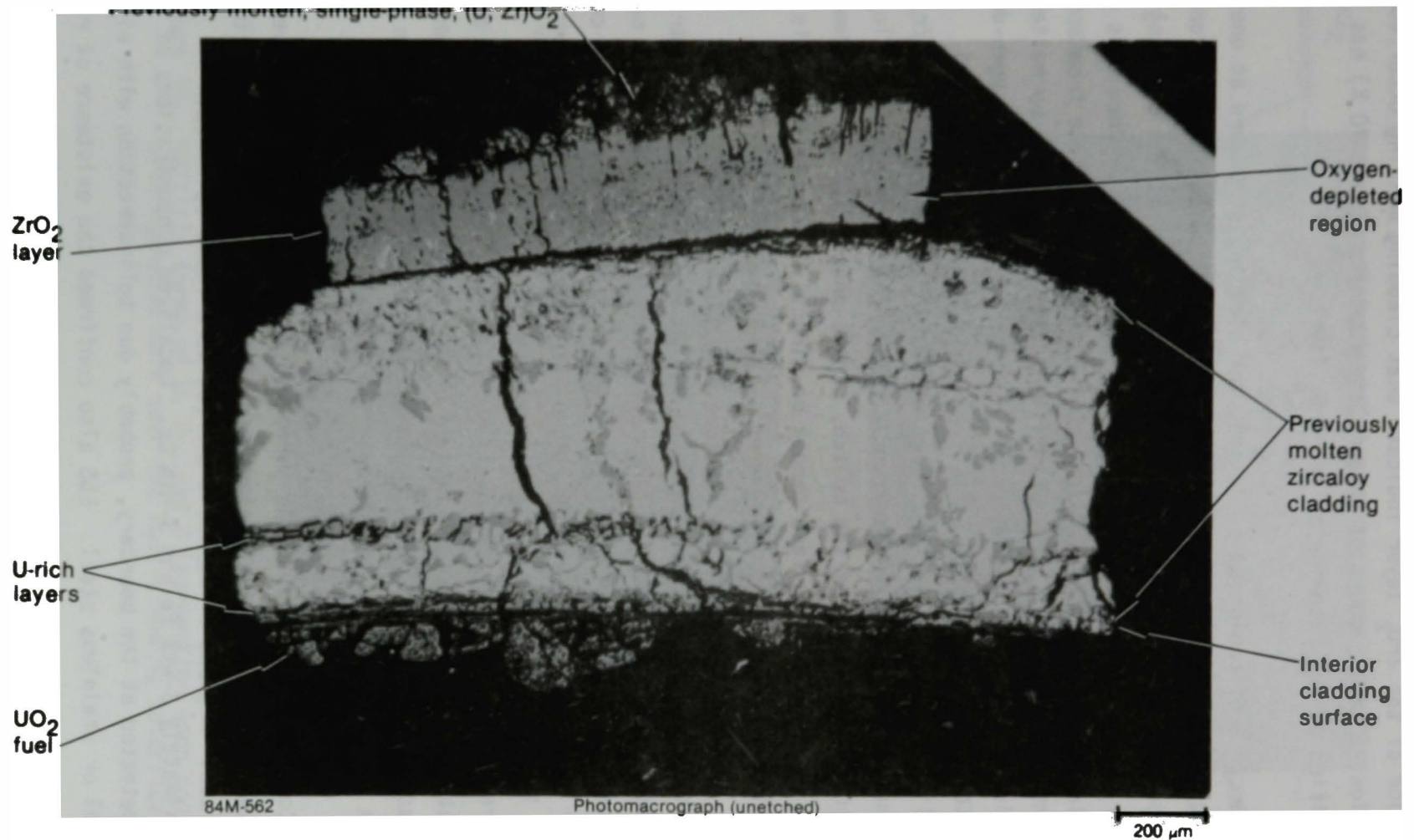
Figure 17. Particle 1E, cladding fragment with adherent fuel and once-molten mixed ceramic.
