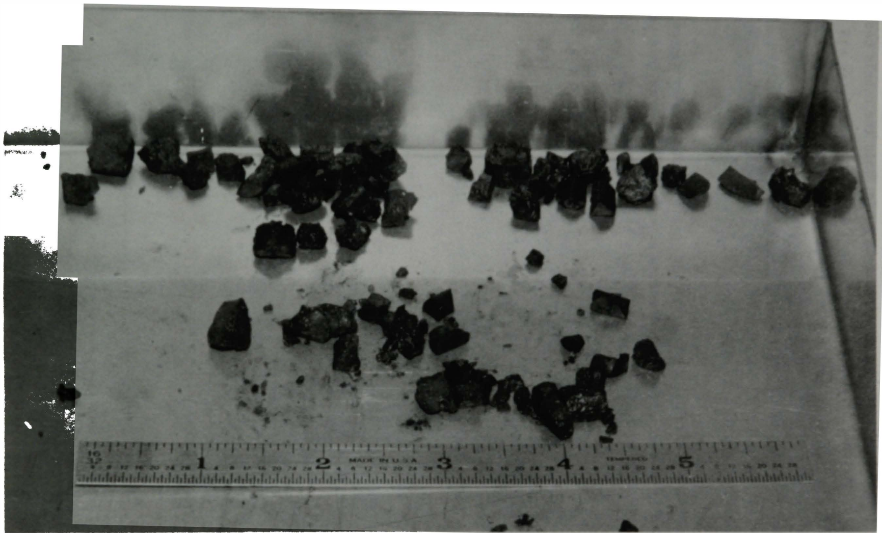
Figure 9. Photograph of Sample 5 which was obtained from 3 in. into the debris bed at the E9 core location.
